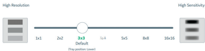
Fig 11. The CCD detector of ImageQuant 800 imager allows for on-chip binning. You can easily change default settings (5×5 for upper and 3×3 for lower tray position in chemiluminescence mode) using the slider. Low binning levels improve the resolution and high binning leads to shorter exposure times.
