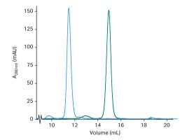
**Fig 9.** Overlay of two chromatograms for analysis of a papain-digested IgG antibody using Superdex 200 Increase 10/300 GL. Blue chromatogram corresponds to intact mAb and green chromatogram to Fab fragment.
