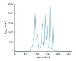
Fig 3. High-sample load (500  $\mu$ L) separation of a mixture containing seven proteins on Superdex 200 Increase 10/300 GL.
