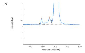
**Fig 8.** Analysis of monoclonal mouse IgG<sub>1</sub> antibody aggregates using Superdex 200 Increase 10/300 GL. (A) Chromatogram without magnification. (B) Magnified chromatogram showing details of aggregates, dimer, and monomer peaks.
