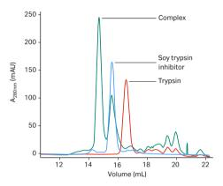
**Fig 11.** Monitoring protein complex formation by analysis on Superdex 200 Increase 10/300 GL. Green chromatogram shows the complex formed between trypsin and soybean trypsin inhibitor. Blue chromatogram shows the soybean trypsin inhibitor peak. Red chromatogram shows the trypsin peak. The complex migrates fast, elutes early, and is shown as a large, green peak.
