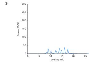
**Fig 4.** A small volume (20 μL with a total of 370 μg protein) of a sample mixture containing seven proteins was separated on (A) Superdex 200 Increase 3.2/300 column and (B) Superdex 200 Increase 10/300 GL column. Both graphs show the same scale for UV detection.
