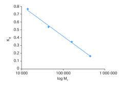
**Fig 2.** Selectivity curve for Superdex 200 Increase resin. The steep slope implies high-resolution separation of proteins in the M range 10 000 to 600 000.
