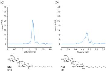
**Fig 10.** Rapid screening of detergents using Superdex 200 Increase 5/150 GL. Purified recombinant membrane protein CE07 was run in a column equilibrated with (A) DDM, (B) UDM, (C) DM, and (D) NM.
