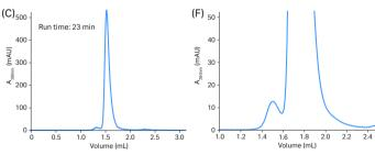
**Fig 5.** Effect of flow rate on cycle time and resolution of mAb monomers and dimers using Superdex 200 Increase 5/150 GL. (A) Run at a flow rate of 0.6 mL/min, resulting in a 6 min separation time. (B) Run at recommended flow rate 0.45 mL/min, resulting in an 8 min separation time. (C) Run at 0.15 mL/min, resulting in a 23 min separation time. D, E, and F are amplifications of A, B, and C chromatograms. For detection, absorbance was measured at 280 nm.
