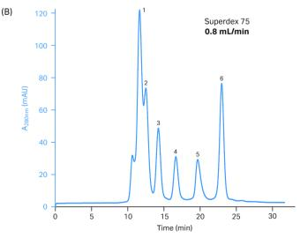
**Fig 4.** Chromatograms showing high-resolution SEC at 0.8 mL/min of a mixture of six standard components on (A) Superdex 75 Increase 10/300 GL and (B) Superdex 75 10/300 GL. Note that increased resolution gives higher peaks, with higher concentrations. In the comparison here shown, the resolution improvement with the new generation column was 40% to 120%, with the largest improvement for the higher-molecular weight proteins.
