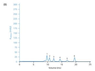
Fig 7. A small volume (10  $\mu$ L with a total of 110  $\mu$ g protein) of a sample mixture containing six components was separated on (A) Superdex 75 Increase 3.2/300 and (B) Superdex 75 Increase 10/300 GL. Both chromatograms show the same scale for UV detection.
