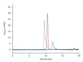
**Fig 10.** Overlay chromatograms of analytical SEC on a Superdex 75 Increase 10/300 GL column. Transcription factor (green) and adaptor protein (red) were separately analyzed. A mixture of the proteins was also analyzed (blue), showing interaction under the conditions used. Image and experimental data are published with permission from Drs. Annika Rogstam and Claes von Wachenfeldt, Lund Protein Purification Platform (LP3), Department of Biology, Lund University, Sweden.
