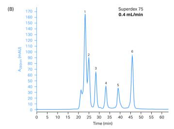
**Fig 5.** Chromatograms showing high-resolution SEC of a mixture of six standard components on (A) Superdex 75 Increase 10/300 GL at 1.5 mL/min and (B) Superdex 75 10/300 GL at 0.4 mL/min. Note that approximately the same resolution was achieved with a 3 to 4 times faster separation using Superdex 75 Increase 10/300 GL.
