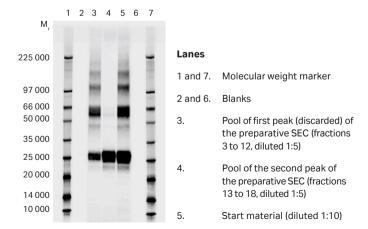
**Fig 9.** Analysis of samples from the preparative SEC purification. SDS-PAGE separation of fluorescent prestained samples on an 8% to 18% gel using Amersham™ PhastSystem™ electrophoresis unit. The system allows automatic scanning of the gel in its run position.
