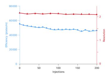
**Fig 3.** Example of results from a study with 200 IgG injections, including harsh CIP procedures after every 10<sup>th</sup> run (1.5 column volumes of 0.5 M NaOH). Efficiency test conducted every 10<sup>th</sup> run after CIP (blue). Resolution determined every 20<sup>th</sup> run after CIP by separation of ovalbumin and carbonic anhydrase (red).
