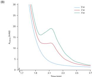
**Fig 11.** Monitoring of size-homogeneity changes of proteins during storage (0, 2, and 4 weeks) using Superdex 75 Increase 5/150 GL for rapid analyses of two purified proteins. In (A), higher molecular weight variants were detected, whereas in (B), degraded products were observed. The area under the curves for the much larger main peaks (not shown) decreased over time, corresponding to the area-increase seen for the small heterogeneity shoulders in (A) and (B).
