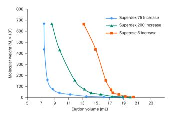
**Fig 2.** Elution volumes for globular proteins of various molecular weights on Superdex 75 Increase 10/300 (blue), Superdex 200 Increase 10/300 (green), and Superose 6 Increase 10/300 (orange). Note! The whole fractionation range of Superose 6 Increase is not covered in this diagram.
