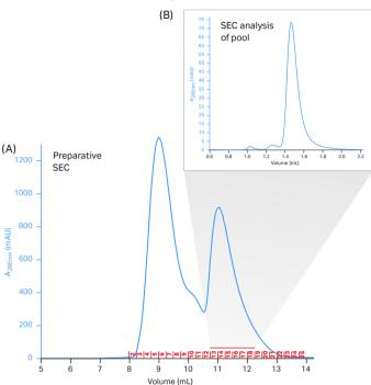
**Fig 8.** (A) Preparative SEC purification of a partially purified and oligomerized histidine-tagged protein. With rapid SEC analysis of fresh fractions (not illustrated), it was revealed that fraction 13, but not fraction 12, was sufficiently size-homogeneous to be included in the pool. The final pool (fractions marked with red bar) contained approximately 5 mg of target protein. (B) SEC analysis of the final pool.
