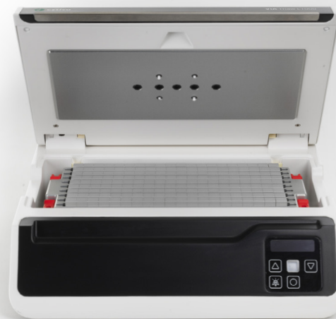
Fig 2. VIA Thaw™ L1000 with thawing tray removed to show the flexible bed.
