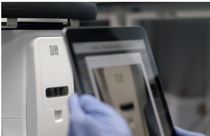
Fig 6. Chronicle eSOP tool records processes, chain of custody, and chain of identity. Image shows bar code reading function within eSOP capturing the unique identity of a shipper unit.
