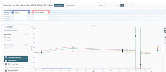
Fig 13. Example of an Interactive run . Each cycle contains an analyte injection (variable concentration) and a regeneration step. The full data set (7 cycles) was then fitted to a 1:1 model in Biacore™ Insight Evaluation Software (data not shown). (Analyte: beta2microglobulin. Ligand: Anti-beta2microglobulin amine coupled to Sensor Chip CM5).
